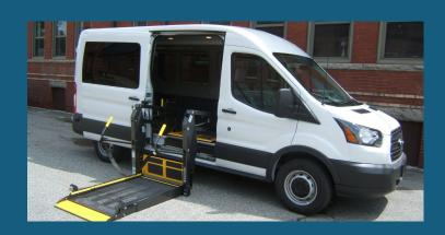
All National Van Builders Wheelchair Accessible vans are custom-built to your specifications and are fully FMVSS, ADA and Ford QVM compliant. Models include Ford Transit in 130", 148" long and 148" extended wheelbase, medium and high roof with available side or rear lift and customized seating plans to meet your specific needs.
