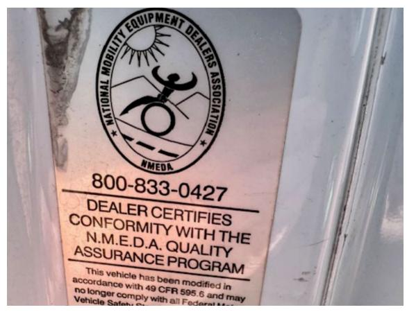
49 CFR 595.6 Identification for Vehicle Modifier to Enable a Person with Disability to Operate or Ride as a Passenger. In this case, covers the addition of the wheelchair lift
